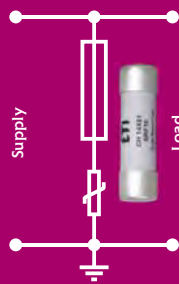
SRF (surge rated fuse)
